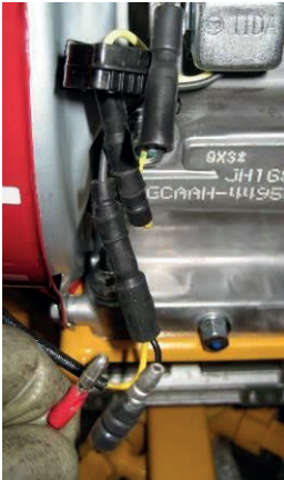
1 DISCONNECT THE BLACK WIRE FROM THE SPARK
