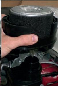
2 REMOVE THE AIR FILTER
