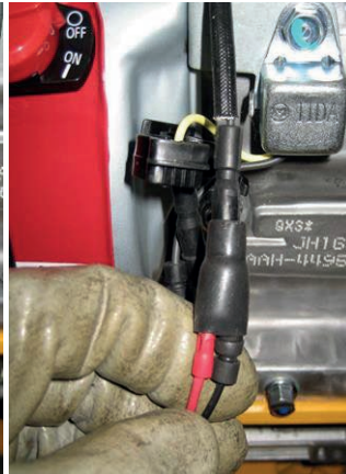
2 CONNECT THE RED CABLE WITH THE MOTOR CABLES
