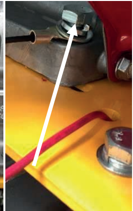
3 CONNECT THE EARTH GROUND TO THE MOTOR SCREW
