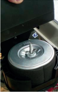
1 REMOVE THE AIR FILTER COVER
