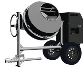
6. Allow the concrete mixer to rotate for 2.5 minutes before using the concrete.
