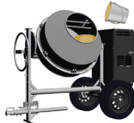
5. Conclude by incorporating the sand and the remaining water.
